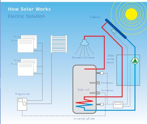
Note: Pilot wire interface unit needed for towel rail and immersion heater
