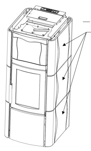
5. starting from the bottom, place the tiles on the iron hooks. Do the same on the other side of the oven (NB the lateral tiles are the same)
